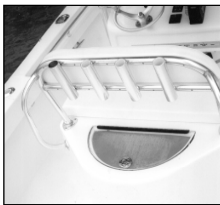
Left: The SeaCraft boasts a clean deck layout, with recessed hardware. Above: A clear livewell lid helps some baitfish survive longer. Crew standing in the cockpit will appreciate the waist-high grabrails on the leaning post.
